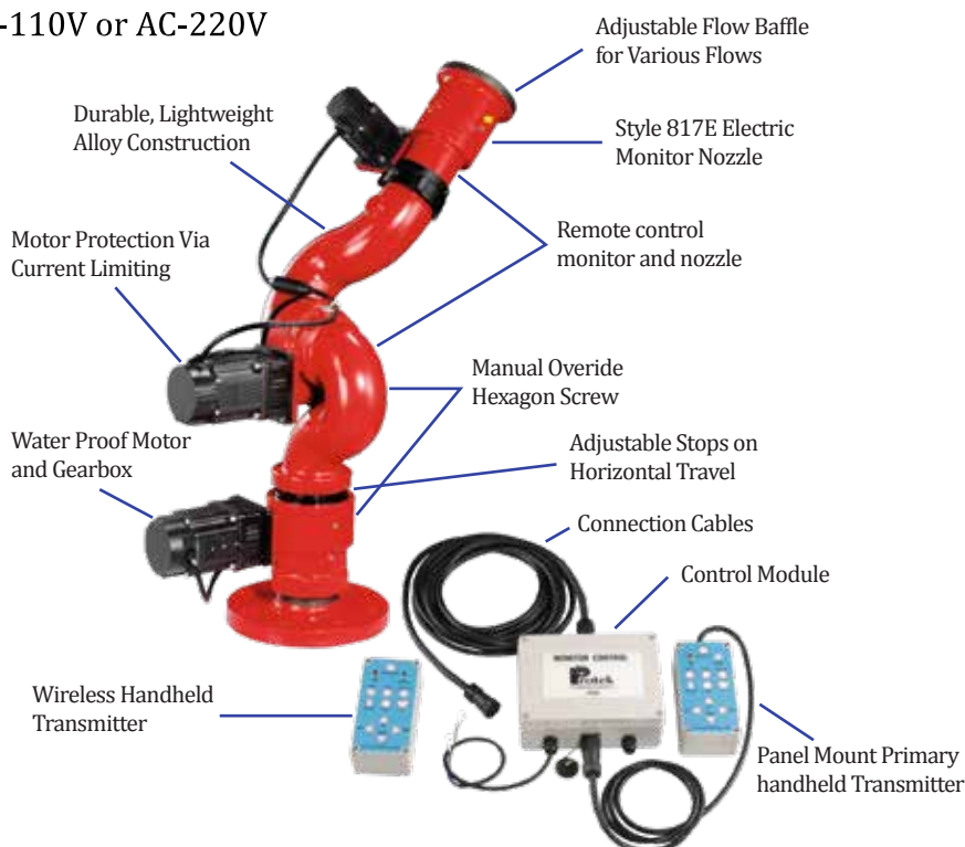
Style 933 monitor shown with standard accessories: Style 817E nozzle, control monitor, connection cables, primary transmitter and wireless transmitter
