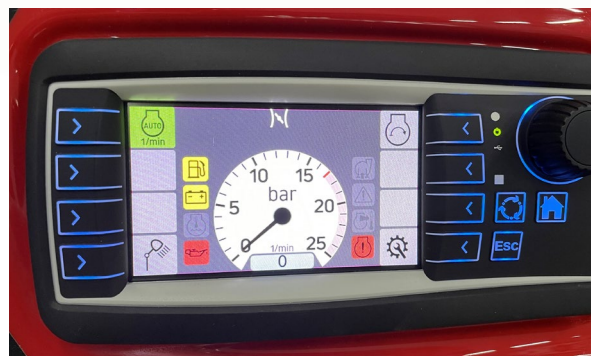
Self-illuminating color display with rotary control for speed adjustment and pump pressure control, as well as a QR code for the online user manual
